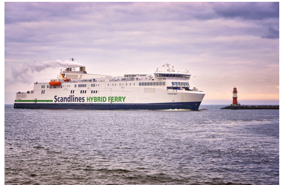
Scandlines ferries combine traditional diesel power with electric batteries. Photo: Adobe Stock
