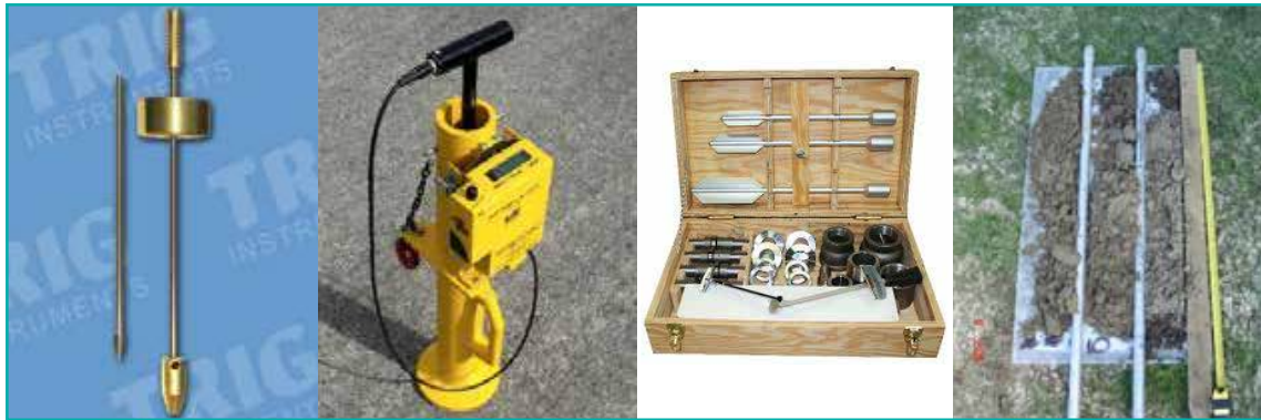
Figure 14. Hand-Held Site Investigation Tools
