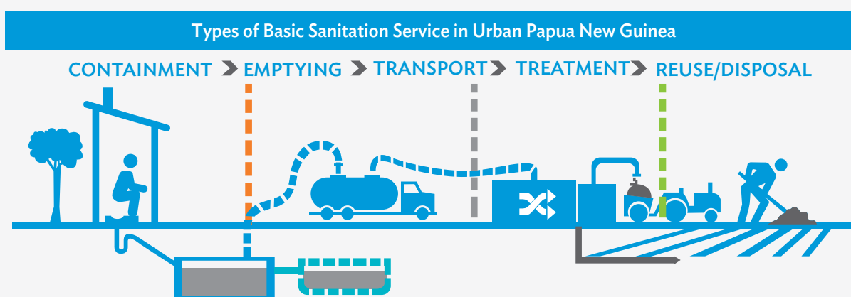
Figure 3: The Sanitation Service Chain
