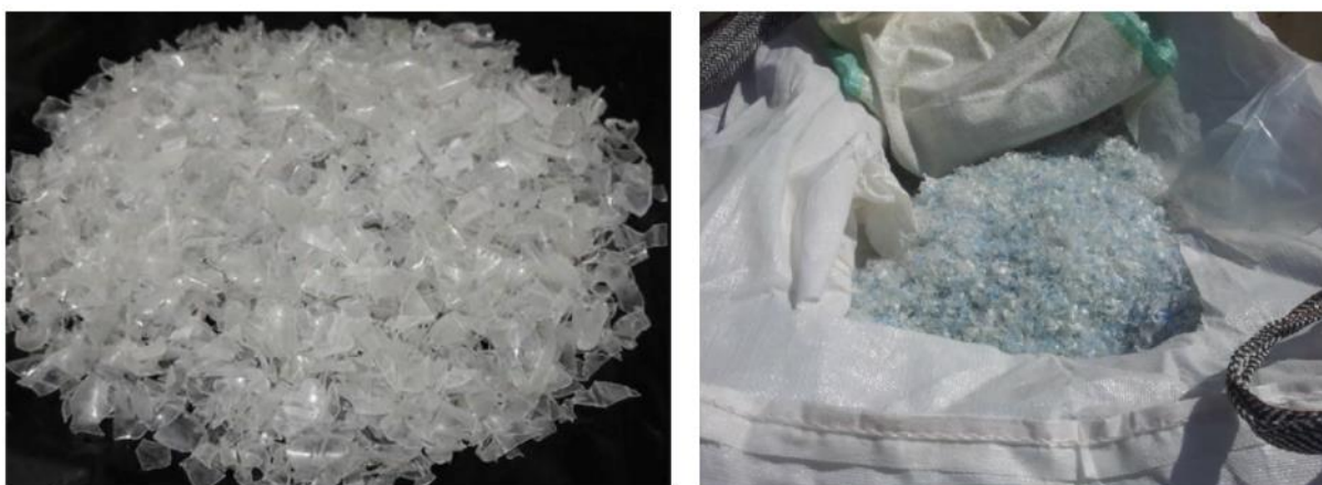
Figure 21 Example of Hot Washed and Flaked PET
