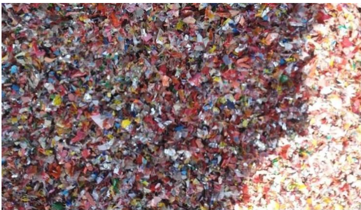
Figure 23 Example of Hot Washed and Flaked Plastic Film
