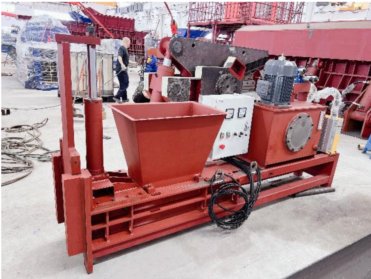
Figure 8 High-Compression Aluminum Can Compactor
