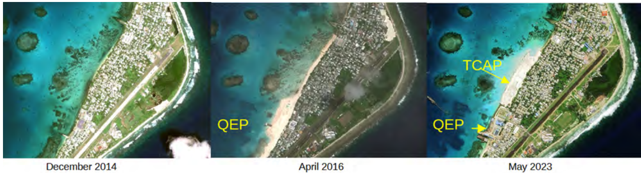
Figure 74: The Progressive Reclamation of the Lagoon Shoreline Adjacent to Vaiaku, Fongafale Island
