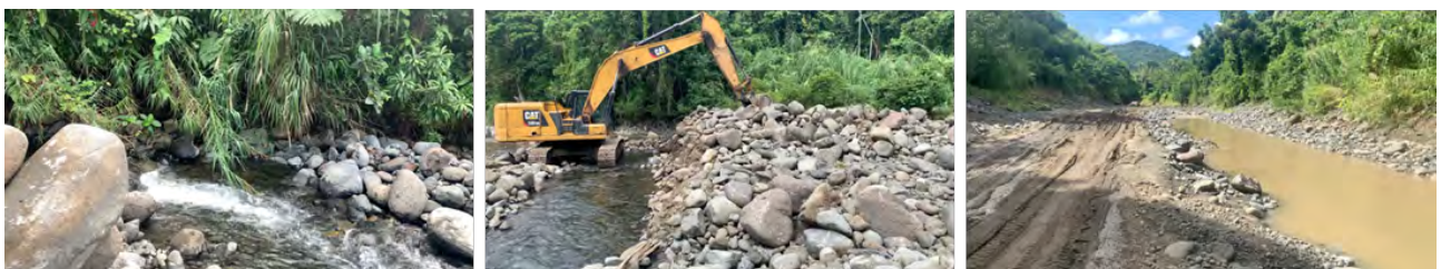
River gravel extraction site in Fiji. Photos show: a) before mining; b) during mining; and post-mining sites (photo credit: Daniel Franks, 2022).
