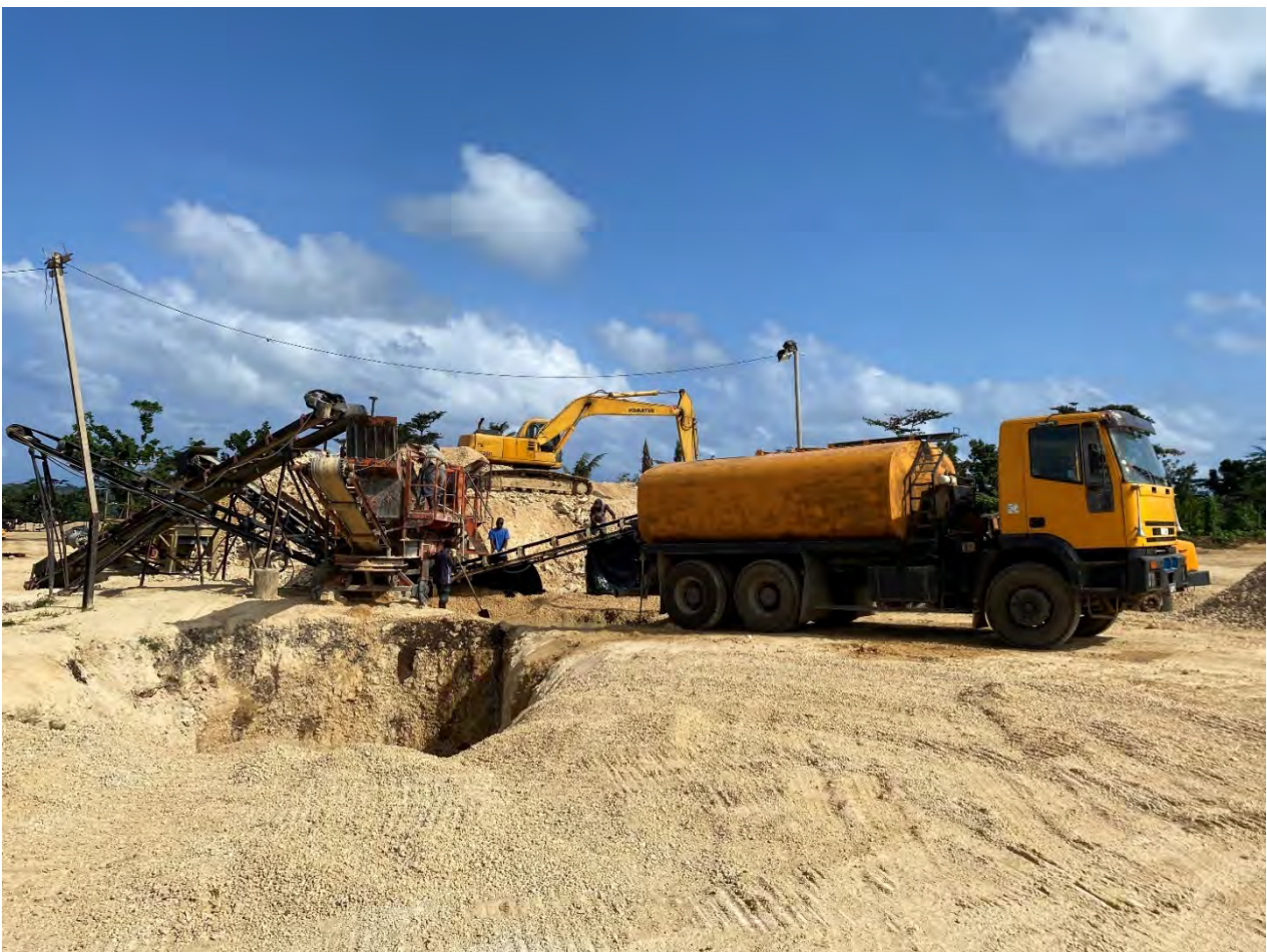
Figure 82: Workers Washing Crushed Limestone Aggregate at a Quarry in Efate
