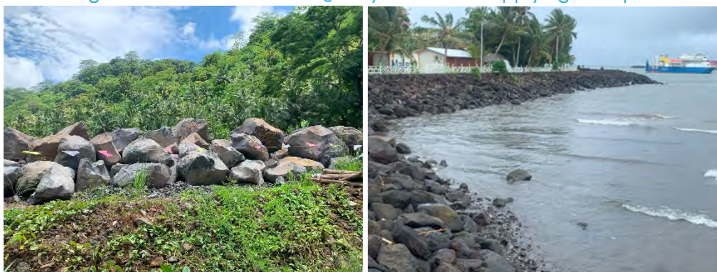
Figure 94: Large Basalt Boulders from Quarry in Samoa Supplying the Apia Port Project
