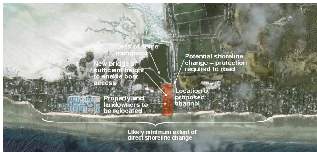
Figure 13: Location of proposed alternative Temaiku channel and summary of main issues and impacts.
