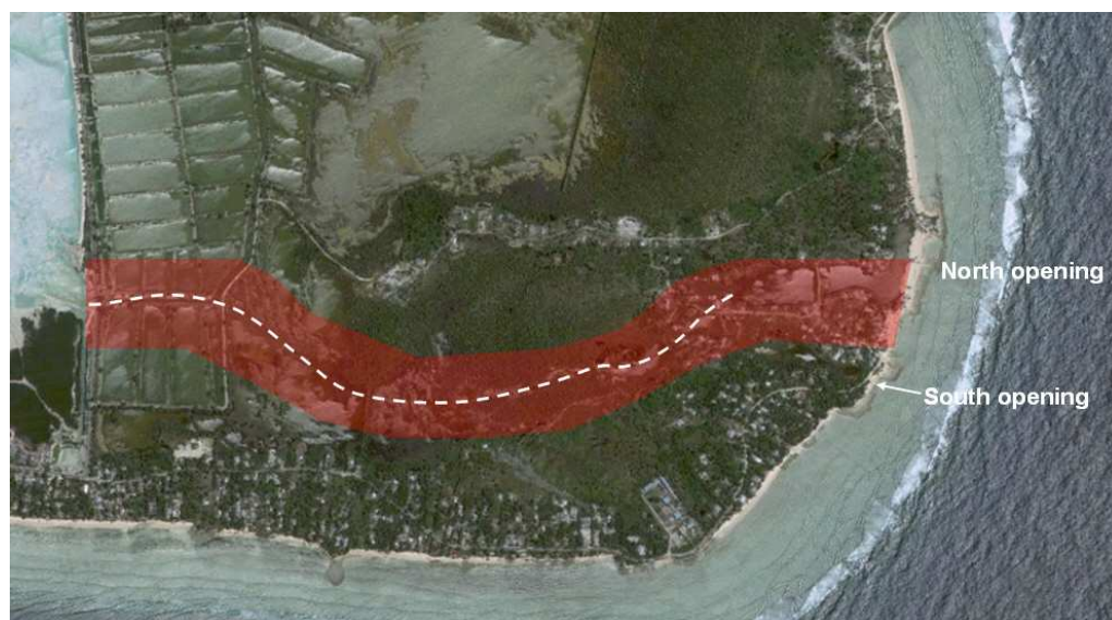
Figure 12: Potential route of a channel at Temaiku (dashed white line) and potential approximate extent of a 200 m wide channel (red shading).
