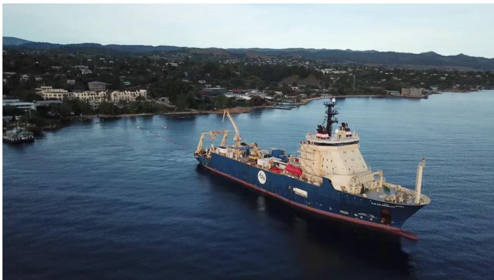
Figure 5. Alcatel Submarine Networks ship laying link to Coral Sea Cable System for the Solomon Islands
