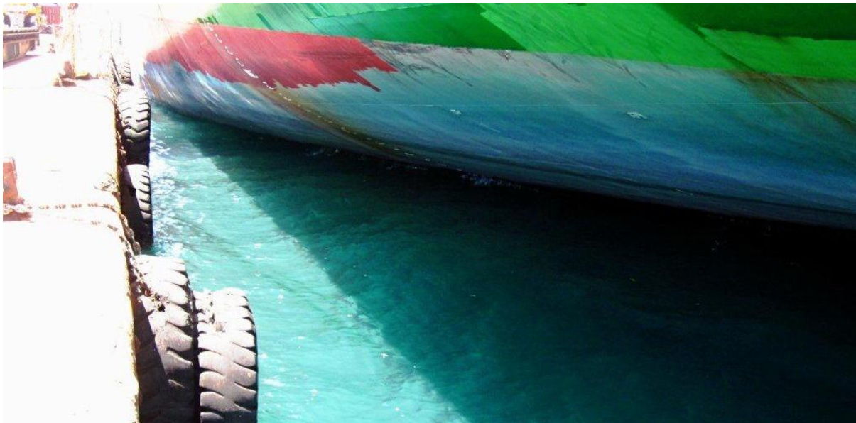
Figure 12 – Used earth moving tyres used as fenders at Main international wharf
