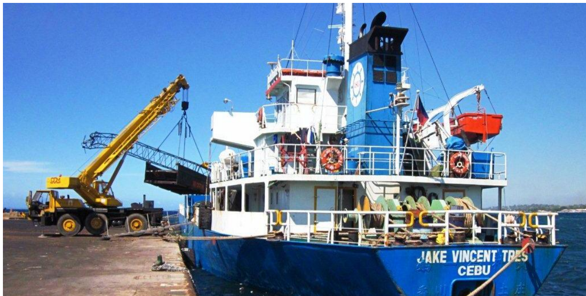
Figure 5 - Bulk copra loading at Honiara using mobile crane and skips
