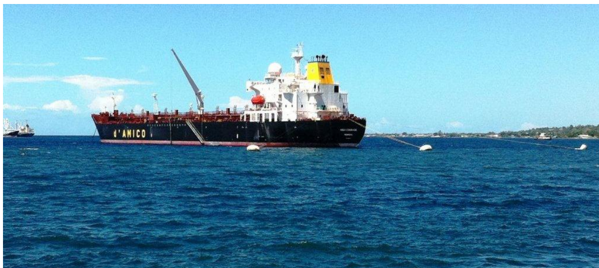
Figure 15 - Tanker at mooring buoys in Honiara discharging petroleum products
