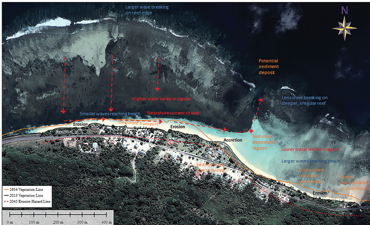
Figure 2-4 Conceptual Model of Coastal Processes Occurring at Manase Beach, Samoa
