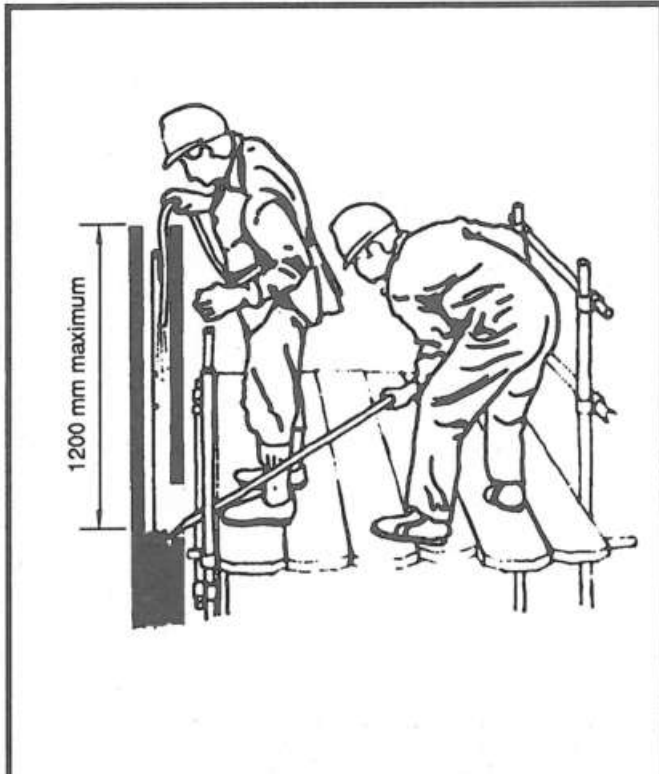
Step 1. Clean out grout space and remove debris. 1200 mm maximum lift when grout space is 50 mm or more. 400 mm maximum lift when grout space is less than 50 mm.
