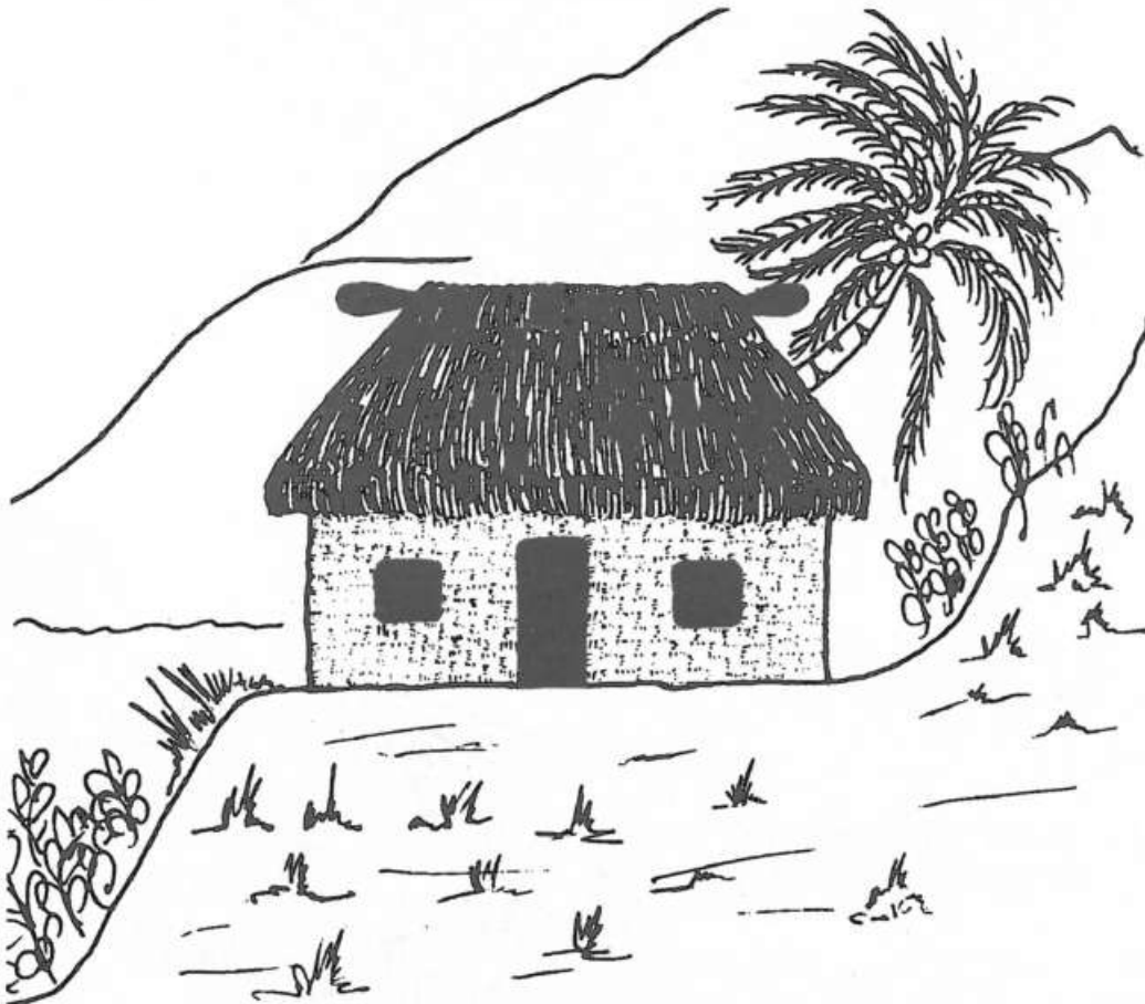
FIGURE F8.8 CUT INTO EARTH IF YOU BUILD A HOUSE ON A STEEP SLOPE
