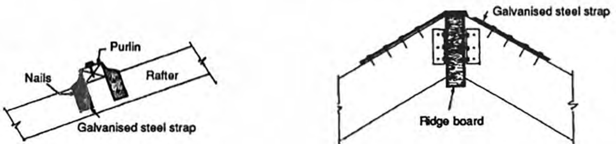
FIGURE E2.7: CONNECTION OF PURLIN
