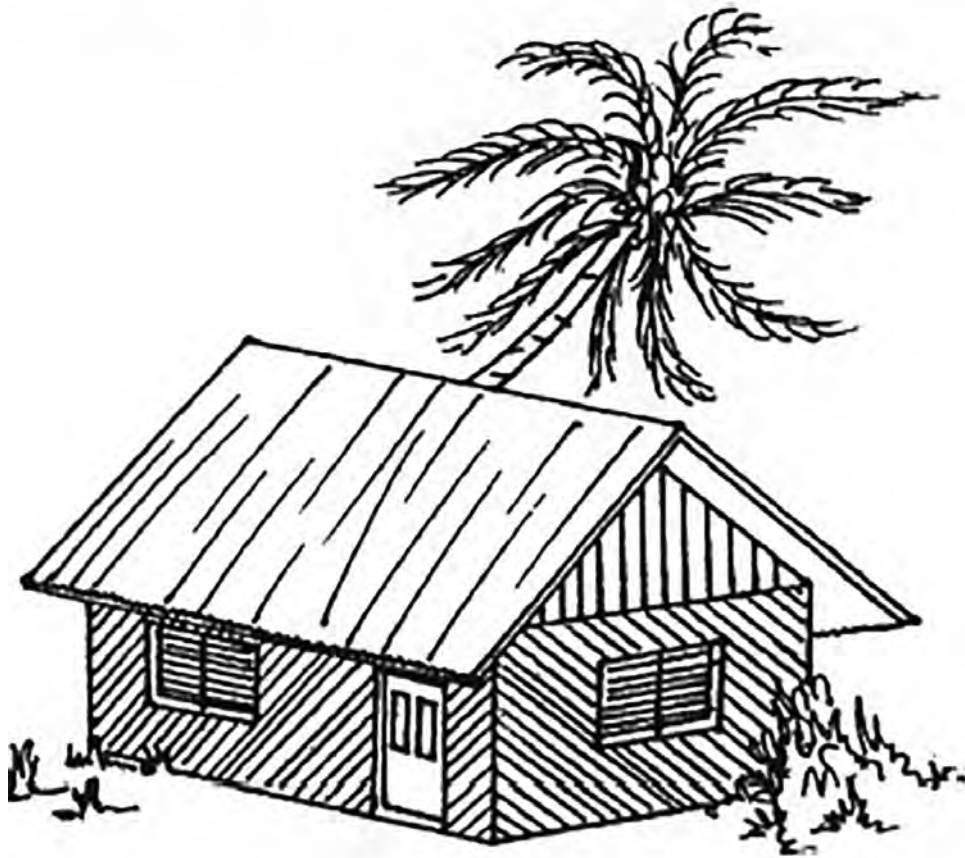
FIGURE F8.19: OVERHANGS MUST BE AS SHORT AS IS NECESSARY
