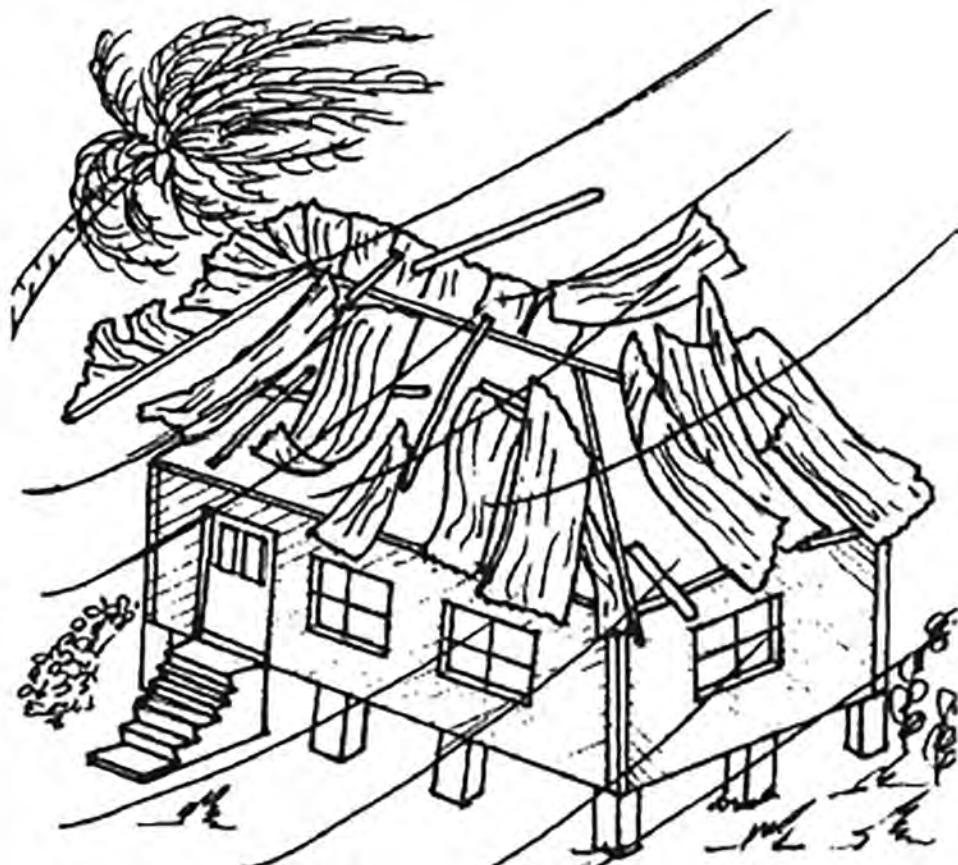
FIGURE F8.2: WINDS WILL BLOW AWAY THE ROOF SHEETING
