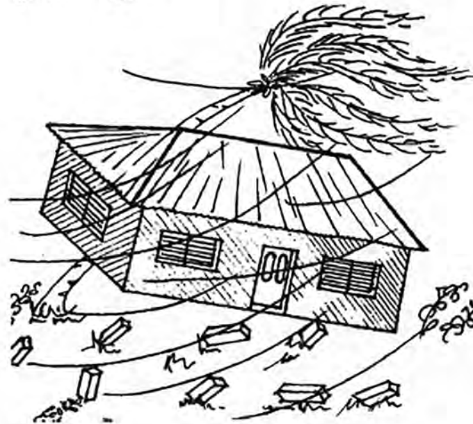
FIGURE F8.13: HOUSE THAT IS NOT PROPERLY TIED DOWN WILL BLOW OFF THE POSTS
