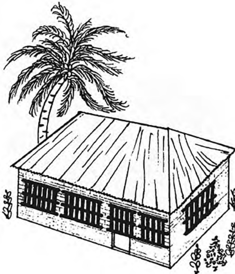
FIGURE F8.17: GLASS WINDOWS AND DOORS WILL BREAK DURING A CYCLONE
