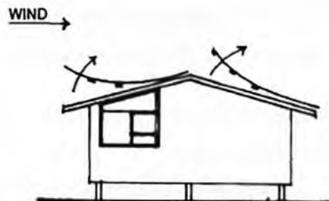
FAILURE: Wind lifts roofing and purlins together REMEDY: Provide adequate fixing of purlins to rafters
