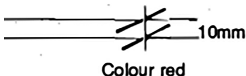
FIGURE NE3.3 - WARNING SIGN FOR PASSENGER LIFTS
