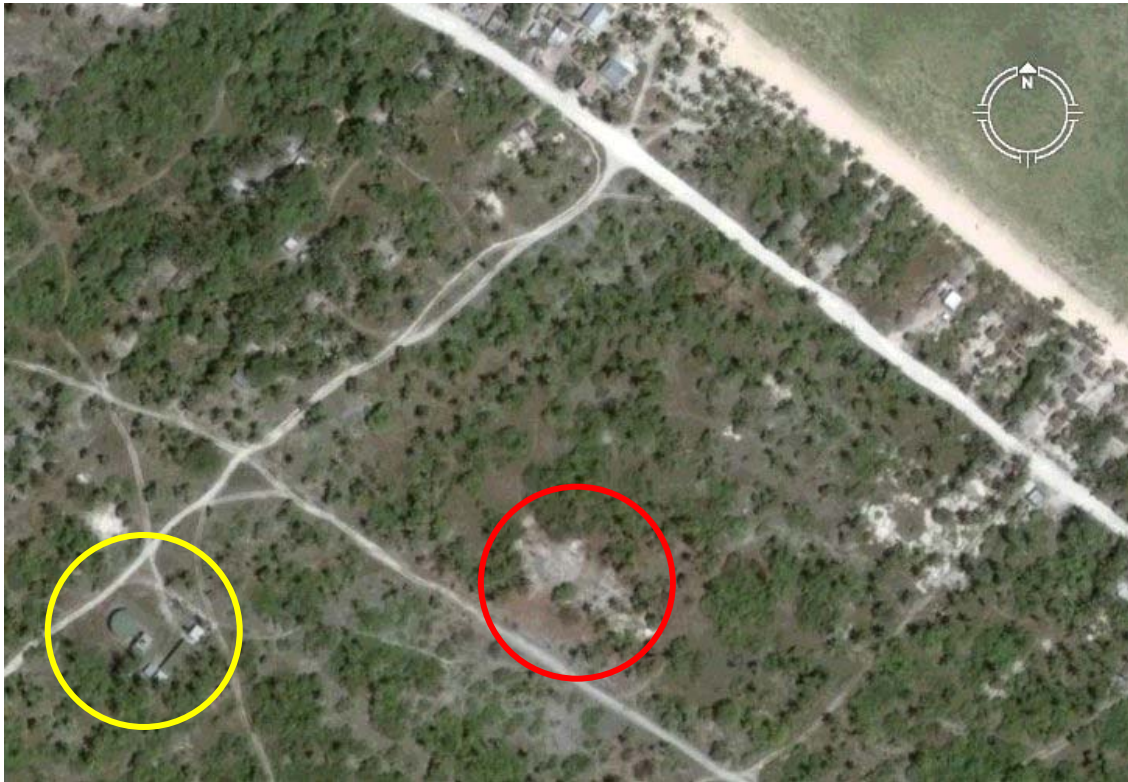
Figure 9. Encroachment of houses onto the Bonriki water reserve across the 50 m boundary road in the northeast. The Bonriki water treatment and pumping plant near the centre of the reserve is circled in yellow and an active cemetery is circled in red (Google Earth).
