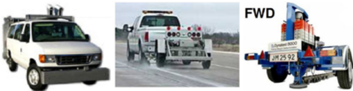
Figure 6-7: Road Evaluation Data Collection through Vehicle Mounted Devices
