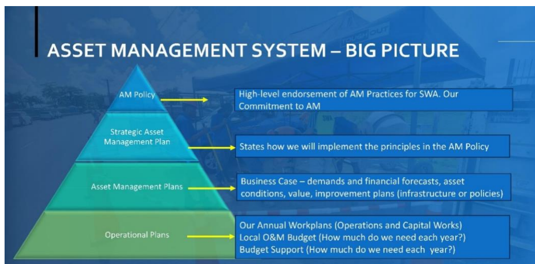
Figure 9: The Samoa Water Authority's Asset Management System
