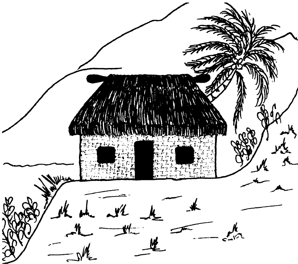
FIGURE F8.8 CUT INTO EARTH IF YOU BUILD A HOUSE ON A STEEP SLOPE
